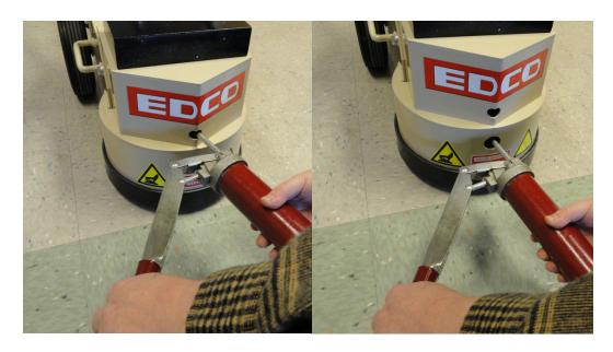
To grease the flange bearings attach the grease gun to the grease fittings as shown in the above photos and give only two (2) pumps on the grease gun weekly. If excessive over lubrication is done grease will leak onto the work surface causing possible damage and wasted cleanup time.
