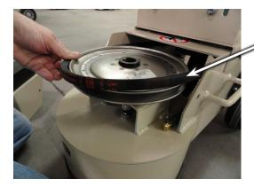
Remove the belt from the motor and driven shaft sheaves as shown in the photo on the left.
