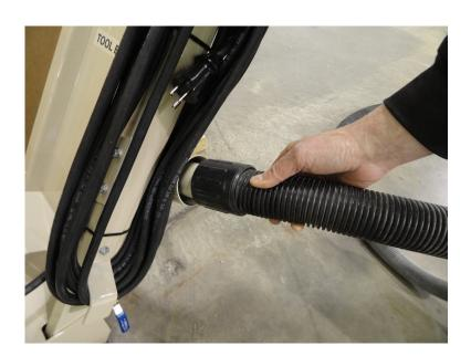
If using a vacuum for dust control attach it to the vacuum port located on the rear of the handle securing it as shown in photo above.
