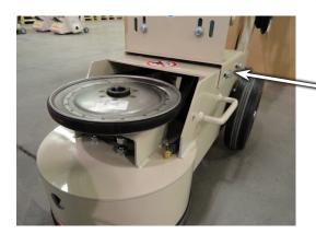
To replace the belt, remove the hood by removing two (2) bolts, one on each side of the machine.
